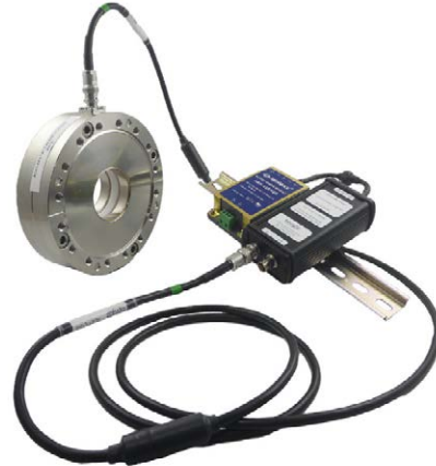
Fig. 3. The ACCT sensor and electronics.
