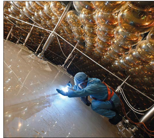
Additional eye Encompassed by photomultiplier tubes, an engineer shines a light inside the acrylic sphere housing JUNO’s liquid-scintillator detector.
