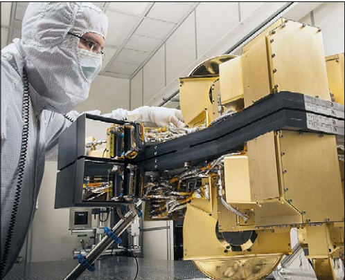
Ultraviolet emission, infrared detection The near-infrared camera of the James Webb Space Telescope.
