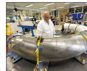
Fusillo, the world's first curved-canted-cosine-theta dipole magnet.
