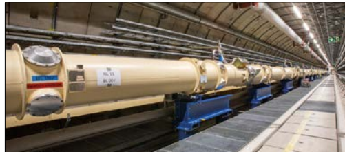
Hunting axions ALPS II repurposes a 250 metre stretch of straightened HERA dipole magnets to search for hidden particles beyond the Standard Model.
