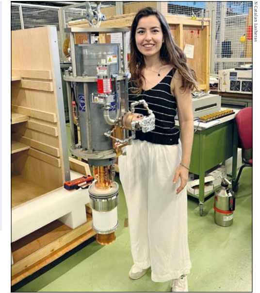
CLIC klystron RF engineer next to the X-band E37113, an industrial klystron by CANON ETD that is being retrofitted with increased efficiency for CLIC.
