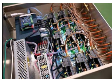
LLRF system with Red Pitaya's STEMLab 125-14 board.
